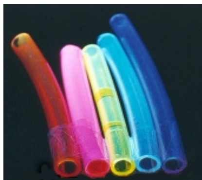
Semiconducting polymers glowing under an ultra violet lamp
