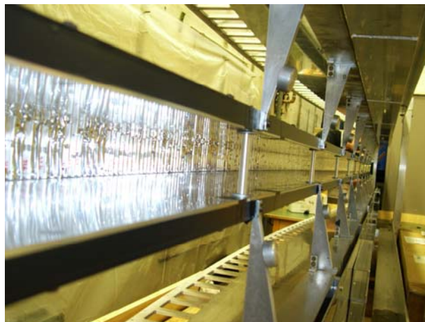
The completely refurbished Glasgow Tagger focal plane detection system.
