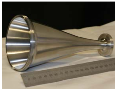
The dissonant vessel that is used for macrosonic wave production, before attachment to driver assembly
