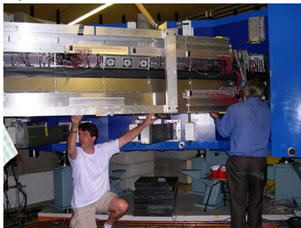
Reinstalling the Glasgow Tagger focal plane detection system. The lighter blue parts of the additional magnet return yoke can be seen.
