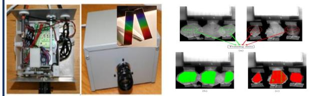
Prototype HCC assembly with internals exposed and as a final compact design. (Insert: LVF)
