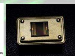
Designed thin film SAW devices
