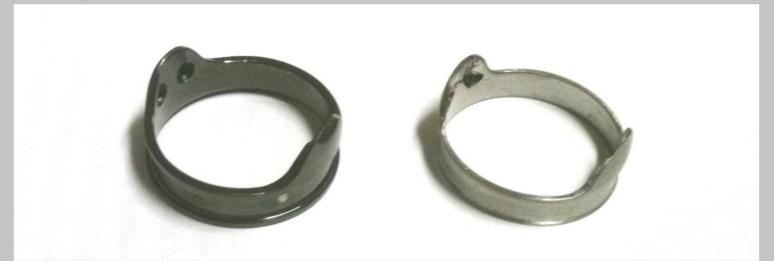
Heart valve rings: right image is the uncoated titanium alloy, left is DLC coated
