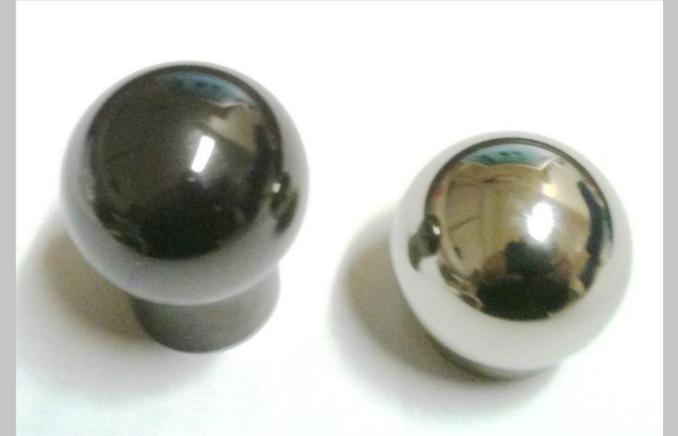
Hip joint test pieces: right image is uncoated Ti alloy, left is DLC coated
