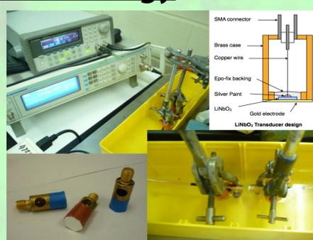
High frequency ultrasound testing in water (top left, bottom right) High frequency transducer design (top right) & devices (bottom left)
