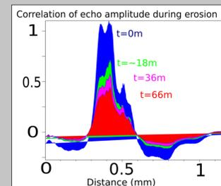
Left: Reflected signal of ultrasound during the erosion of the tooth surface with 80mMol HCL, where a strongly detectable drop in reflection amplitude is observed as the surface becomes disrupted. Note that this change in surface is not detectable at such an early stage with current clinical tools. HCL erosion is biomedically relevant to studies of acid erosion through gastric reflux and bullimia.
