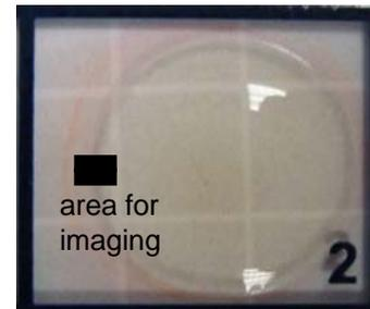
DASPMI entrapped in Gellan Gum analysed using FLIM
