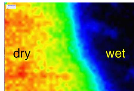
Viscosity changed ~600x moving from dry to wet front
