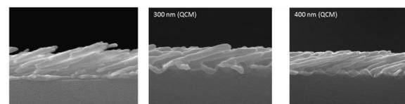
Figure 1 – (left) oblique angle deposition of copper on silicon (100) substrate, no template features mean that nucleation for nanostructures rely on random sites. (middle and right) oblique angle deposition of silver onto polymer templates at varying thicknesses measured *in-situ* by a quartz crystal microbalance.
