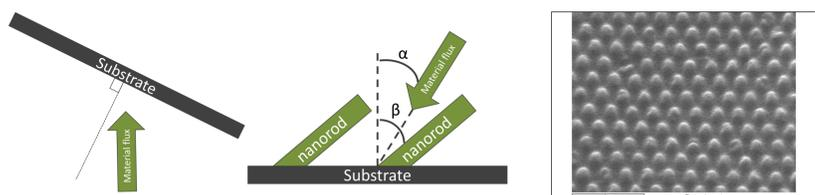
Figure 2 – (left) Brief diagram illustrating the operation of oblique angle deposition and the angles involved when carrying out such depositions. (right) The hexagonal packing structure allows for nanorod arrays to be formed due to the atomic self-shadowing effect at high deposition angles.
