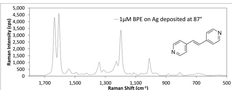
Figure 5 – SERS spectrum of BPE on Ag nanorod array produced by 87° OAD. These arrays produced the best enhancement signal, giving approximately 100,000 enhancement factor.
