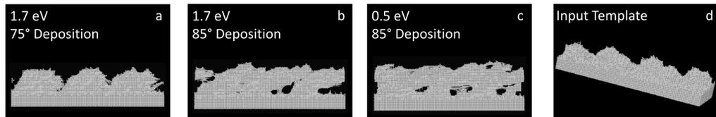
Figure 4 – NASCAM simulations of Ag deposition onto a template surface (d) at lower deposition angles (a) and surface diffusion energy closest to those found in literature (c).
