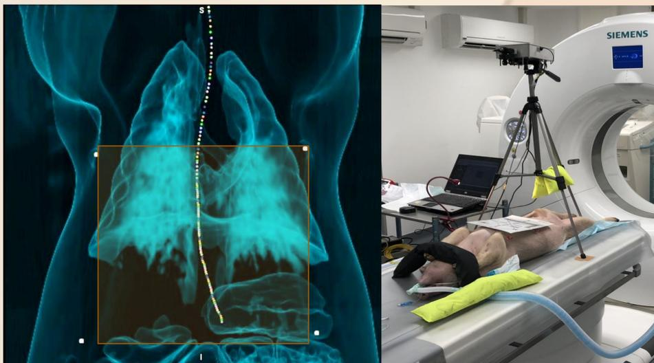
Left: CT Verification Scan, Right: Experimental setup, MegaFrame 32 imaging system placed over the patient, creating an effective field of view of  $\approx 30\text{cm}^2$
