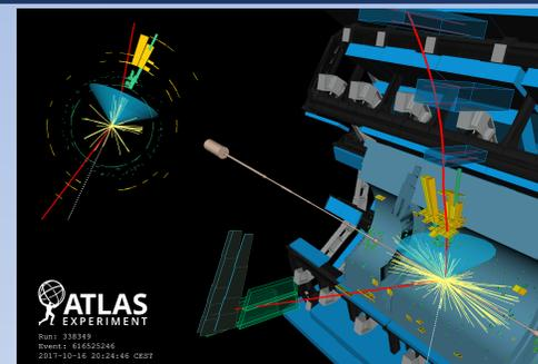
**Figure 1:** A very boosted  $H \rightarrow b\bar{b}$  event display from the ATLAS detector where particles originating from the two b-quarks (green and yellow energy deposits in the calorimeters) have been merged into a single jet (blue cone).
